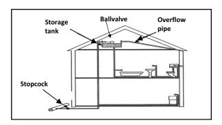
(i) Explain the function of the following parts of the cold-water system shown above:
